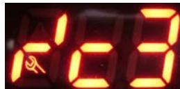
If the condenser probe is installed it is possible to check condenser temperature by means of the parameter **/C3** (calibration or offset for condenser probe)
