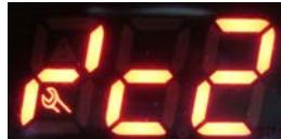
Current evaporator probe temperature is available by means of the parameter **/C2** (calibration or offset for evaporator probe)
