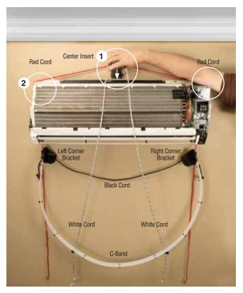
3. Slide Left & Right Corner Brackets under back corners of the unit. Tighten Corner Brackets by pulling Red Cords through the Cord Locks. Secure Corner Brackets together by tighten Black Cord and securing with Cord Locks. ▼
